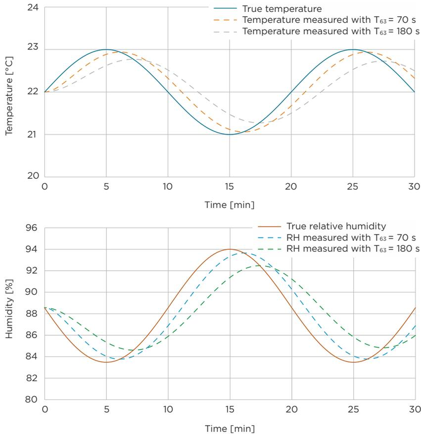
Figure 2. In the upper graph, the dashed lines represent the temperature readings of two instruments with different  $T_{63}$  response times in a slowly changing temperature. In the lower graph, the impact of the temperature measurement error on the relative humidity measurement is shown. The slow stabilization with respect to temperature causes an additional 3 ... 4 %RH error in the relative humidity measurement.
