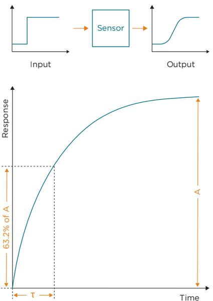
Figure 1. The first order linear time-invariant system
